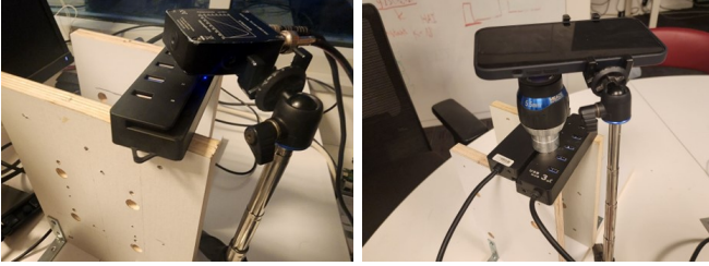
Fig. 3. Recovering a frequency scan using a photodiode (left) and a smartphone (right), by capturing video footage of the power LED of a USB hub.
